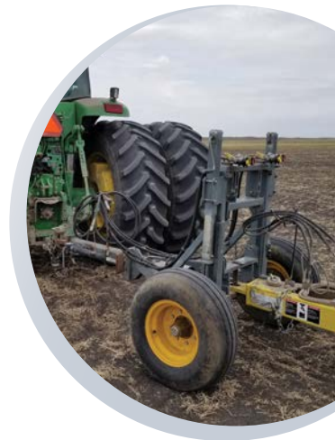
PAMI load cart connected between a power unit and a roller.
