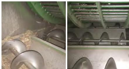
Pay attention to any horizontal augers and the clean grain, and return elevators. Finally, inspect and clean the sieves (Figure 5).
