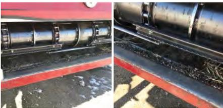
The feeder house (Figure 1) can be a major source of material contamination. Once the feeder house is clean, move to the stone trap and blow out any material that is hanging in there, paying particular attention to any corners where material can adhere to the combine (Figure 2).
