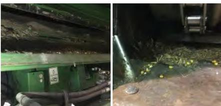
Now it's time to move to the top of the combine and grain tank. When cleaning the grain tank you should always blow the material towards the unload sump. Pay close attention to areas of the hopper such as the auger and areas behind the auger where material can accumulate (Figure 3). Before you move down to the threshing area, blow off the top of the cab. The threshing area, concave and
