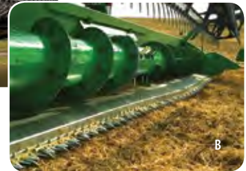
◀ Figure 2. Auger header (A) equipped with an air reel; (B) without an air reel. (Source: PAMI)
