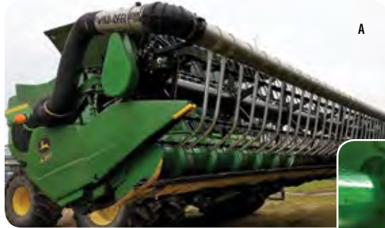
◀ Figure 2. Auger header (A) equipped with an air reel; (B) without an air reel. (Source: PAMI)
