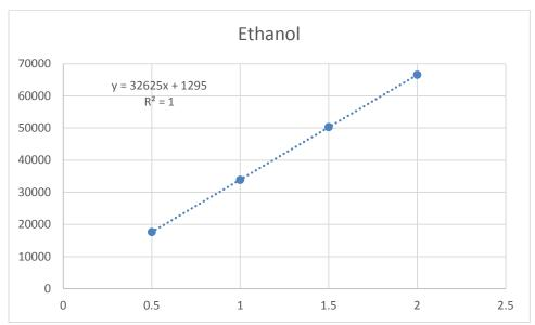
Calibration of the refractive index detector of the Agilent 1100 HPLC system using the Aminex HPX 87H column with 100% ethanol. Conditions were 0.5 mL/minute flow rate in 8 mM  $H_2SO_4$  at room temperature.
