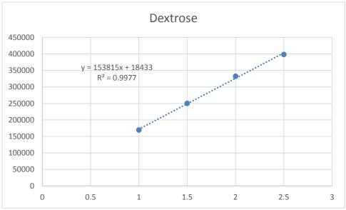
Calibration of the refractive index detector of the Agilent 1100 HPLC system using the Aminex HPX 87H column with dextrose (glucose). Conditions were 0.5 mL/minute flow rate in 8 mM  $H_2SO_4$  at room temperature.
